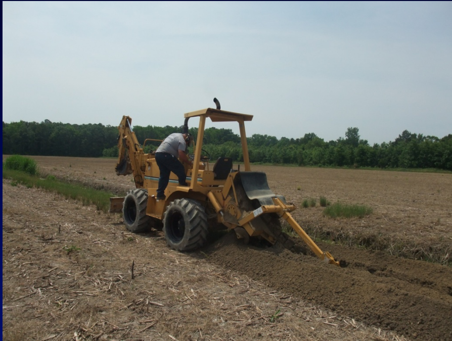
Trencher with one foot wide belt
